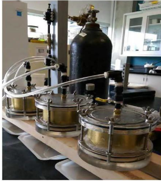
Figure 2. Pressure cells (Tempe cells) used to determine the CRE of tailing mixtures.
