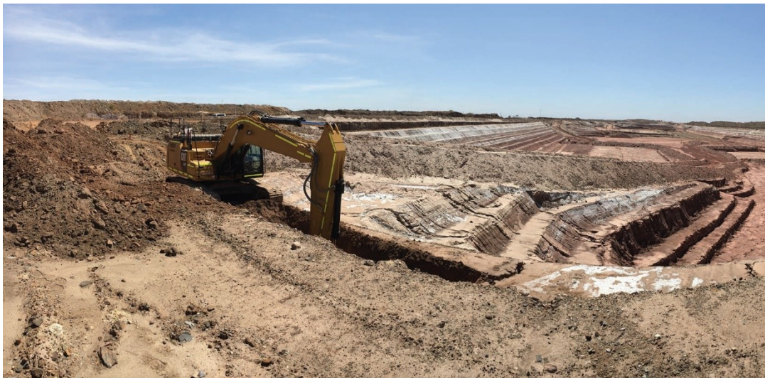
Figure 1. Tailings harvesting operation (adapted from Chapter 8 in SME Tailings Management Handbook).
