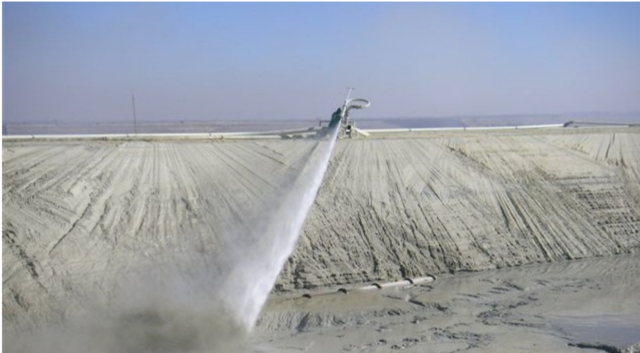
Figure 2. A typical hydraulic tailings remining operation (Boswell et al., 2013).
