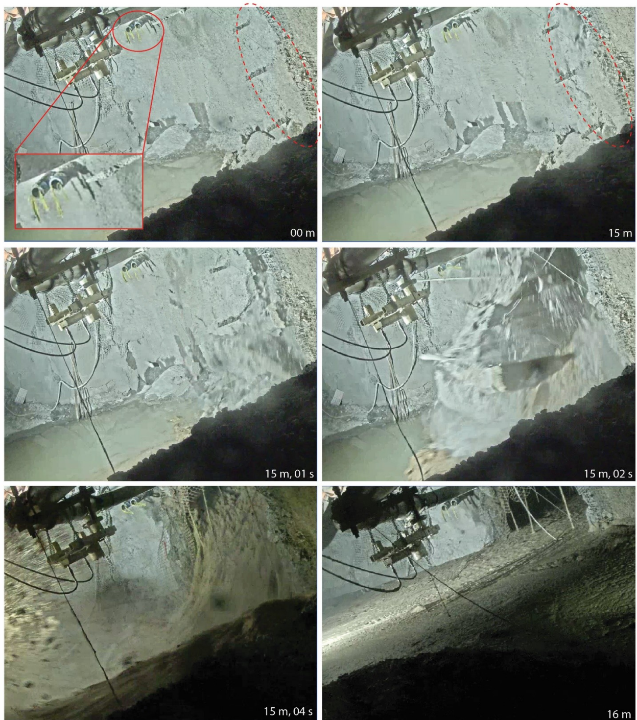
Figure 2. Images showing barricade failure. The solid circle shows breather pipes with flags to indicate air flow, and the dashed circle highlights initial movement.
