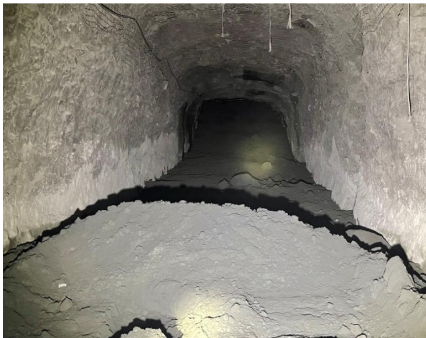
Figure 6: Under-strength paste remobilised into the draw point of adjacent stope after vertical exposure.
