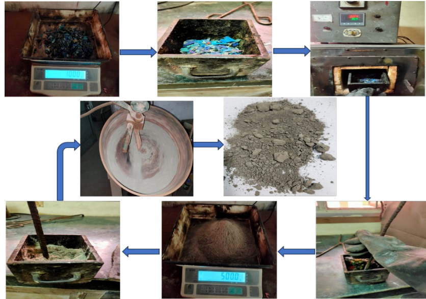
Figure 4. Step-by-step process of SLAs synthesis, starting at the top left image.
