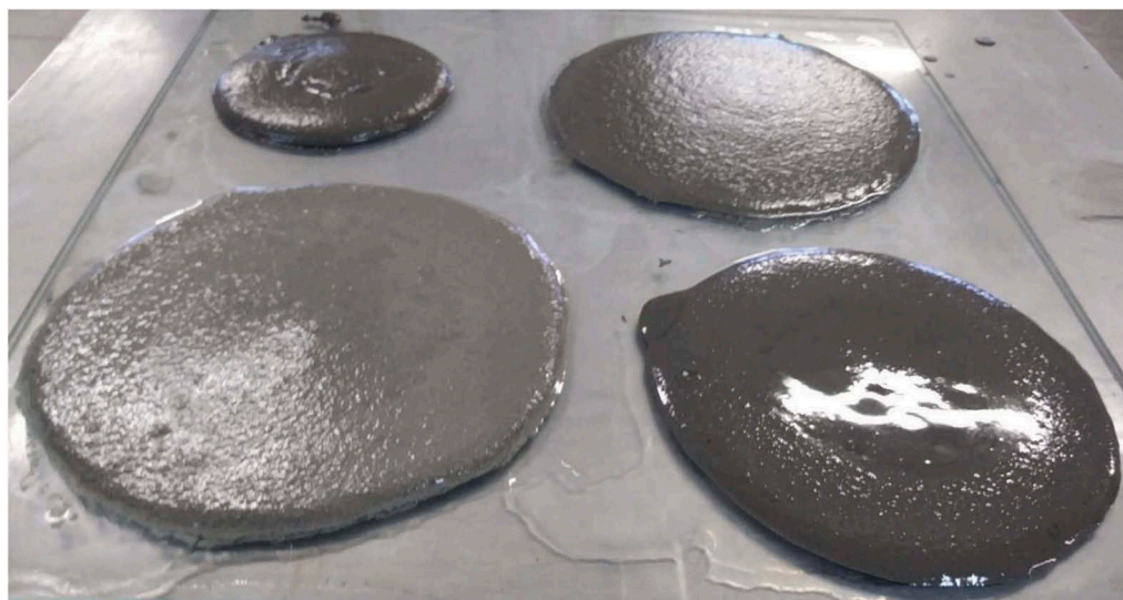
Figure 1. Exemplary flow cakes being a measure of flowability.
