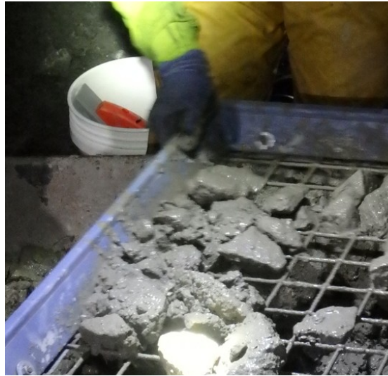
Figure 2. Process of screening two inch plus sized coarse aggregate for screened 6 \times 12 in CRF cylinders.
