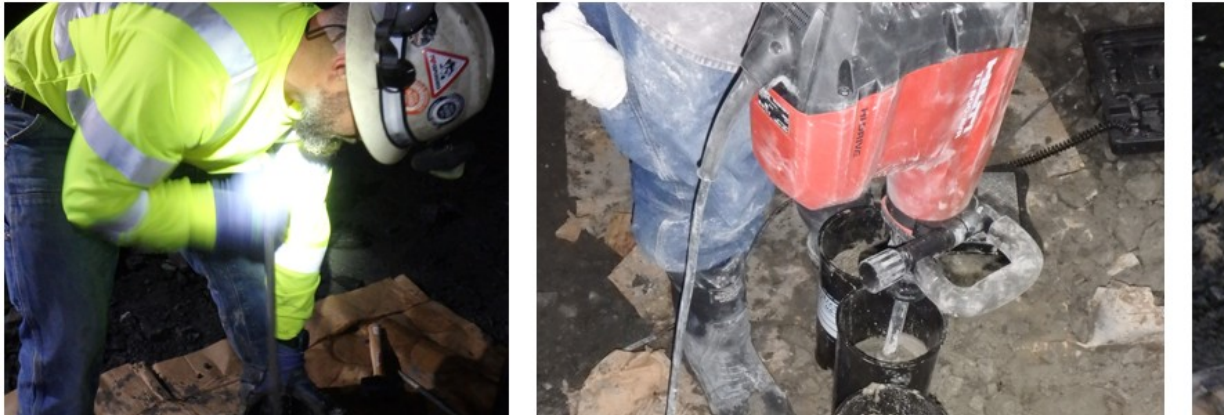
Figure 1. Example of researcher constructing 6 × 12-inch CRF cylinder according to a) ASTM C31, b) ASTM C1435, and c) drop hammer compaction method.
