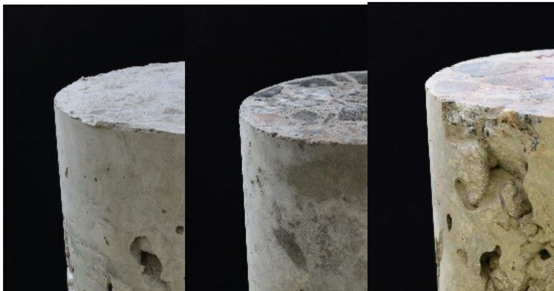
Figure 3. Example of cured, not-screened samples after molds were removed a) ASTM C31, b) ASTM 1435, c) drop hammer compaction method.
