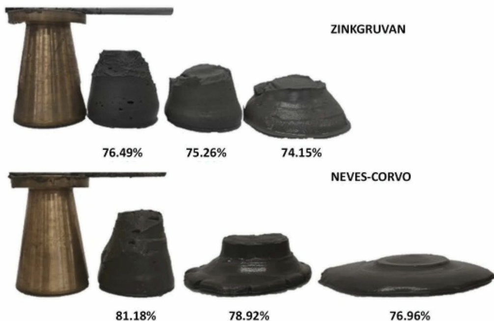
Figure 11. Photographic record of slump tests.
