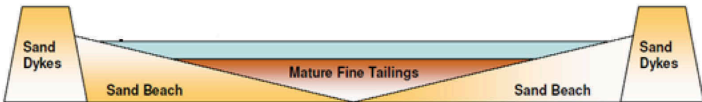
Figure 5. MFT deposition zone in cross-section of TSF.
