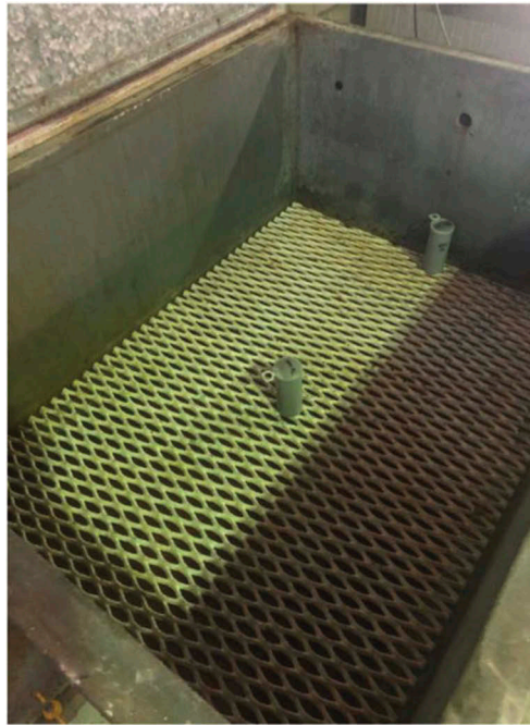
Figure 4. Photograph of curing chamber used in experiments.
