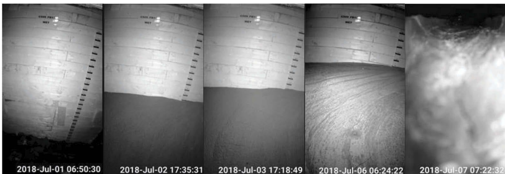
Figure 4. Monitoring paste backfill through remote camera.
