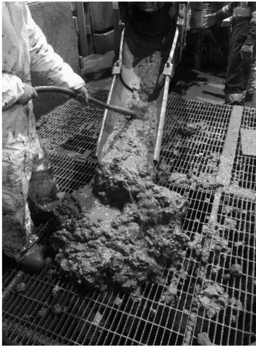
Figure 9. Frozen paste caught on the screen. Source: MineFill Services project database.
