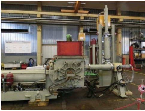
Figure 8. Hydraulic Driven S- Tube Pump with Hydraulic Pulsation Dampening System.
