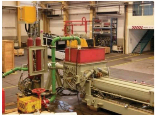
Figure 8. Hydraulic Driven S- Tube Pump with Hydraulic Pulsation Dampening System.
