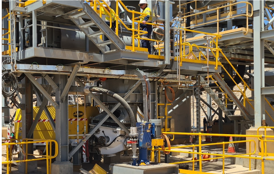
Figure 9: Concrete pump within paste plant.
