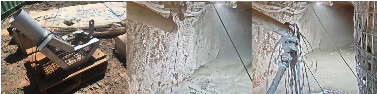
Figure 3. Images showing the catcher when delivered (left), when not engaged (middle), and engaged with CPB flowing (right).
