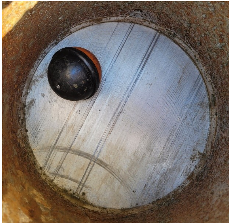
Figure 1. A Piper instrument cluster inside a 200 mm diameter pipe.
