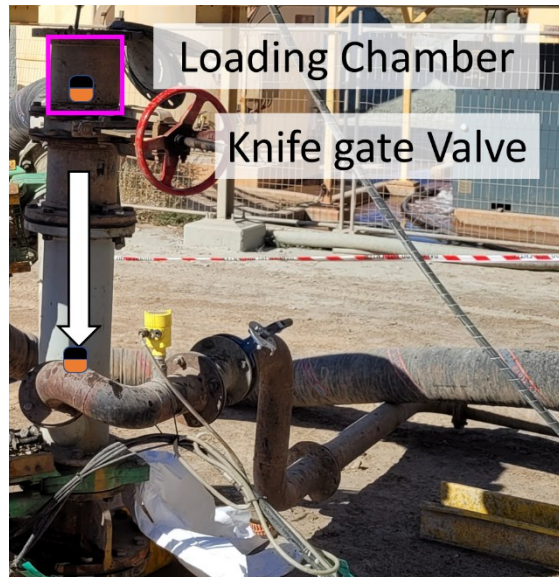
Figure 2. A photograph showing the knife gate valve spool for launching the Piper into the UDS.
