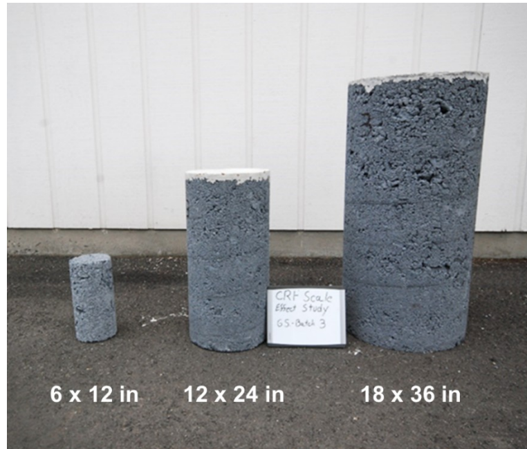
Figure 2. Example of the three sizes of backfill cylinders tested from Batch 3.
