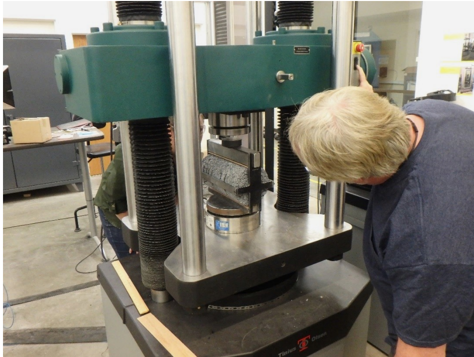
Figure 6. Splitting tensile strength test with a 6×12 in CRF sample.
