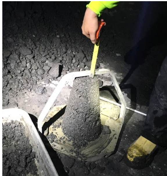
Figure 3. Slump test with CRF mix from Batch 1.
