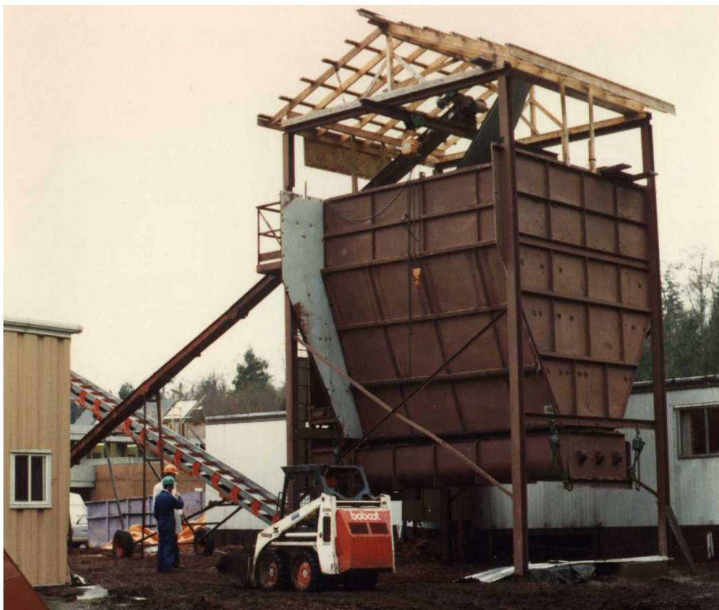
Figure 7. Triple screw auger mounted to adjustable test bin. The test bin geometry, including sloping wall angle, discharge outlet, and bin liner surfaces were adjusted according to the theory for a given material. To explain the plugging in the test bin, the researchers made two key observations on the effects that the feeders were having on the flow of material in the storage bin.
