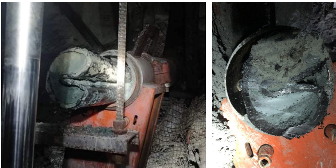
Figure 4. Failed HDPE borehole piping protruding out of level piping leading to a line blockage.
