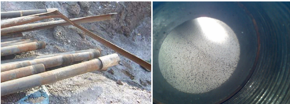
Figure 10. P110 Oil Field ‘casing’ pipe shown completely worn through after 150,000 t of fill (left). ArmorPIPE inspection in same application after 2,000,000 t of fill (right).
