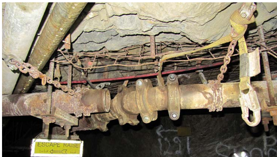
Figure 2. Paste fill pipeline diversion
