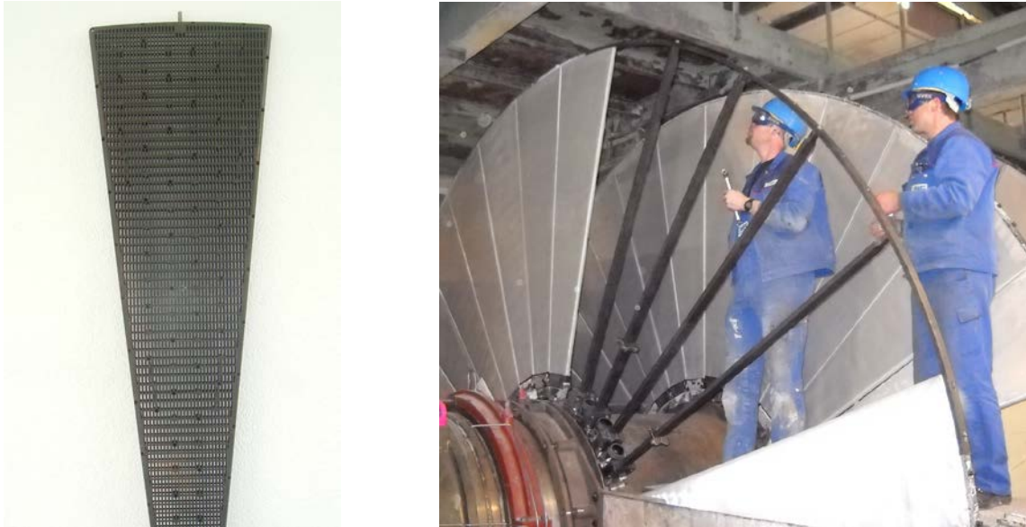
Figure 2. New lightweight snap-on segment of only 12 kg in weight (left), mounting of new segments onto a Spoker Boozer (right)
