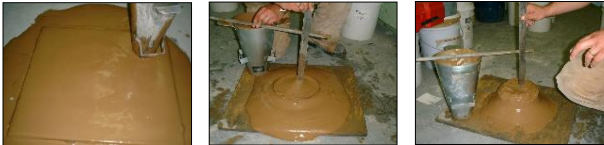
Figure 2. Mixture of solids and water at different densities forming no slump (left), 10 inch slump (middle) and 7 inch slump (right)
