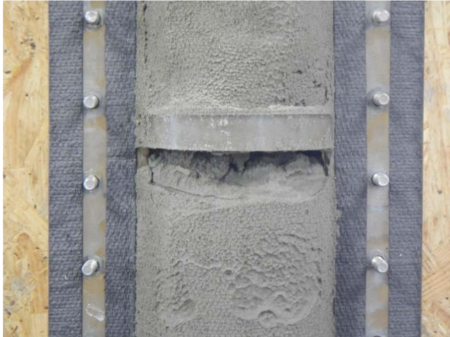
Figure 10. Backfill column separation
