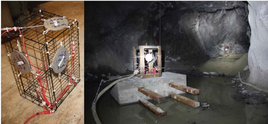
Figure 2. (left) Cages containing instruments are installed in steel cages (right) and bolted onto concrete bases for easy, remote controlled transport. Cage 1 was installed under the brow of the stope, with Cage 2 shown in the center of the stope.
