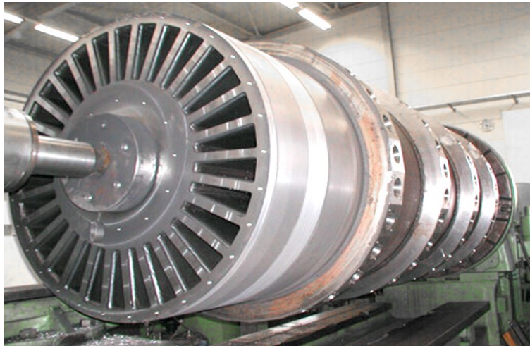
Figure 10. Centre barrel with trapezoidal filtrate pipes
