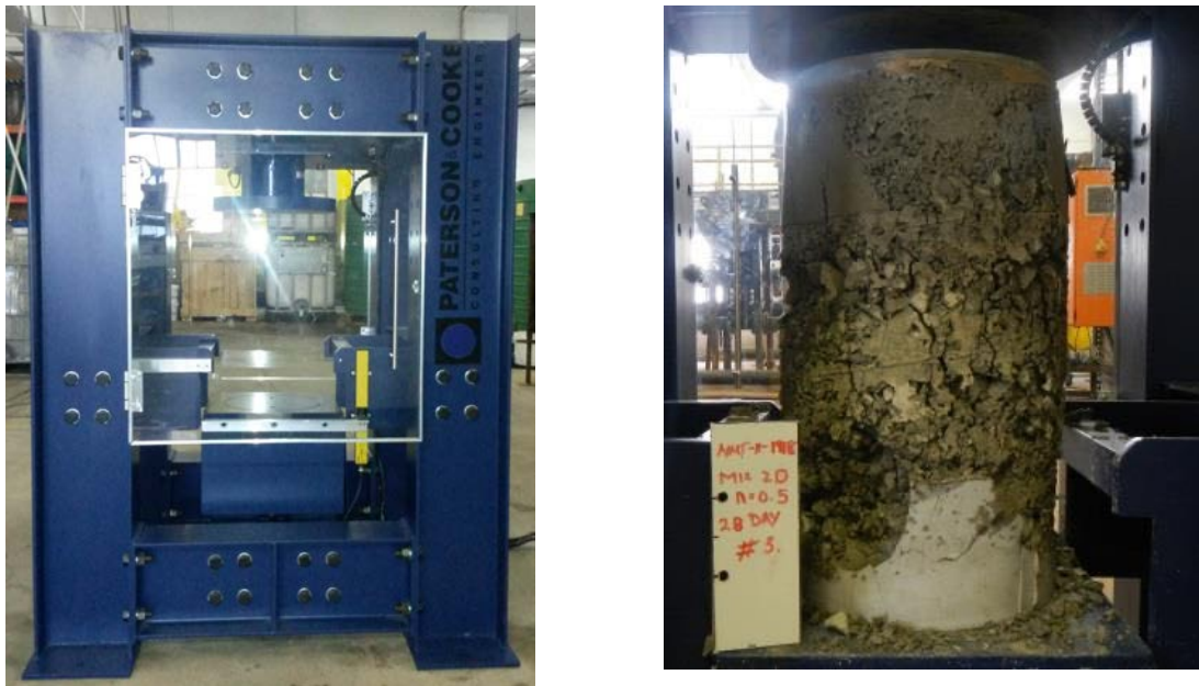
Figure 4. 50 tonne load frame (left) and cylinder being testing (right)
