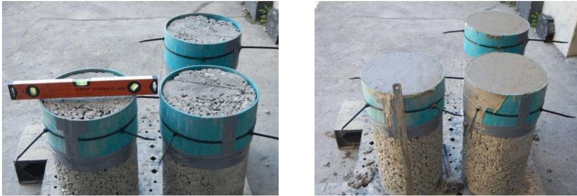
Figure 3. Capping of cylinders; level filling (left) and finished cap (right)
