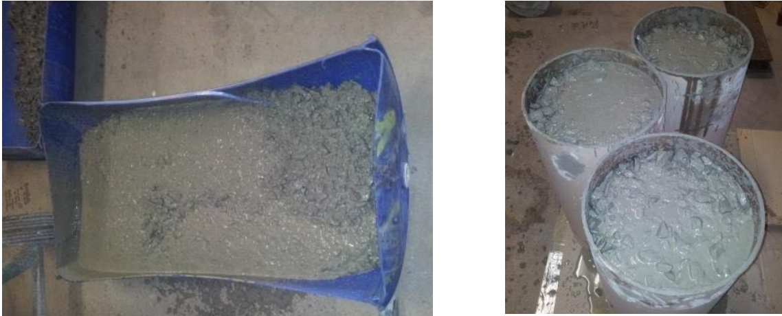
Figure 1. Sample preparation prior to casting cylinders; mixed sample (left) and filled moulds (right)
