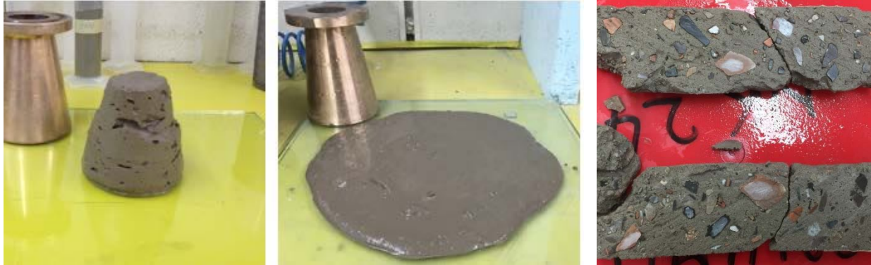
Figure 7. Paste mix from the mortar-cone testing before adding admixtures (left) and after adding 2% Sika® Stabilizer-305 MBF (middle). In the right image, note the very homogeneous distribution of the added crushed aggregates when cutting the cured paste after 28 days.
