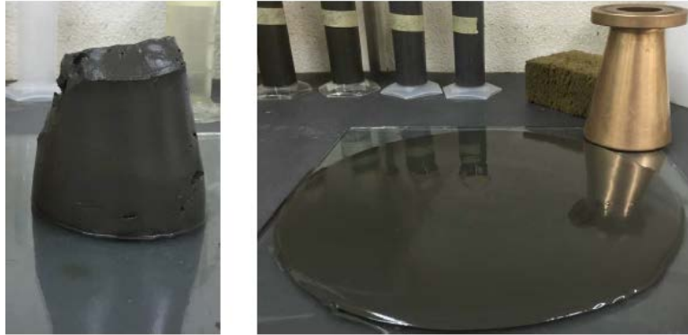
Figure 4. Paste mix from the mortar cone testing before adding admixtures (left) and after adding 1.8% Sika® Stabilizer-302 MBF
