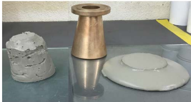
Figure 5. Paste mix from the mortar cone testing before adding admixtures (left) and after adding 3% Sika® Stabilizer-301 MBF
