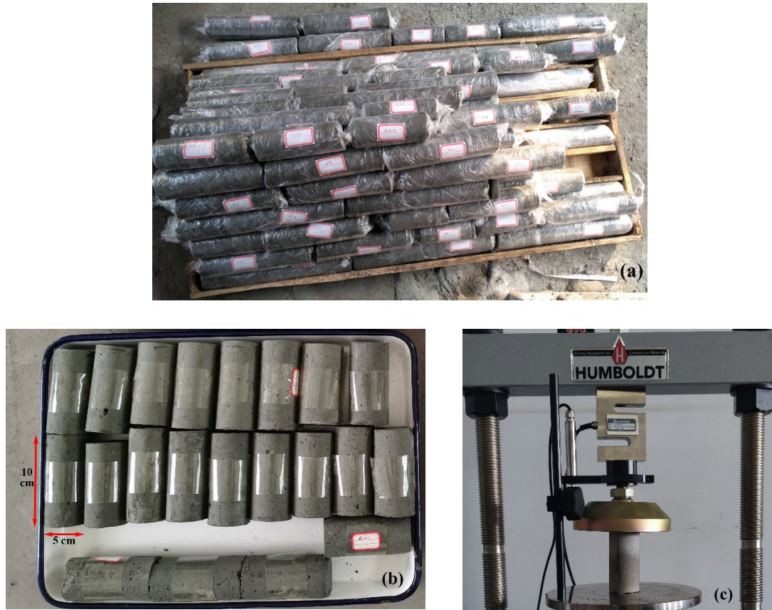
Figure 2. The drilled CTB specimens test process, including: (a) the drilled core backfill mass, (b) UCS testing specimens, and (c) the testing apparatus.
