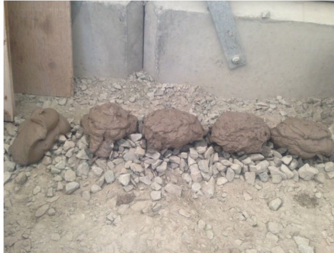
Figure 1. Paste without EBF (left most pile) and with EBF (right 4 piles)
