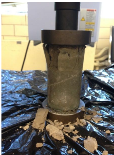
Figure 2. Base (without EBF) paste had broken pieces falling off from the sample after UCS testing was completed
