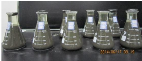
Figure 6. Results of water segregation test for different tailings
