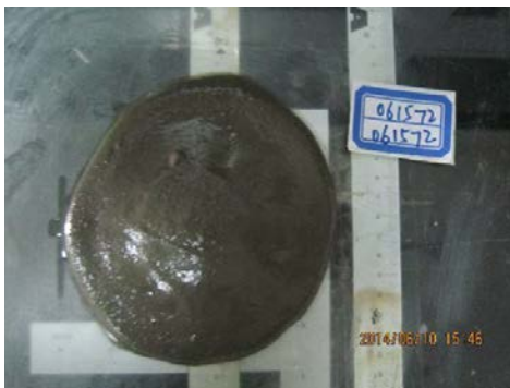
Figure 7. Slump test process and results
