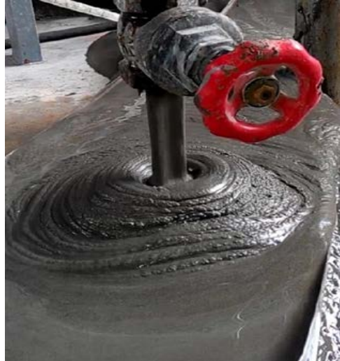
Figure 9. Sand discharging effect drawing of filling slurry for mixed tailings at the filling pipeline sampling mouth
