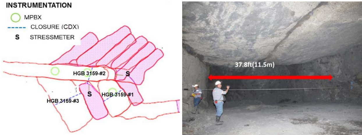
Figure 7A and 7B. Plan map of HGB 3159 level, showing MPBX, CDX, and stressmeter locations. Photo of wider undercut area using tape extensometer for horizontal convergence measurement (HGB 3159-#3).
